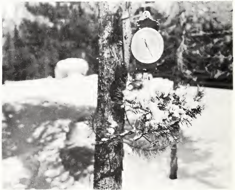
Figure W-7. -- The snow on this lodgepole pine branch was reduced by evaporation from 8 ounces to 3.5 ounces in 2 hours and 40 minutes. None of the snow was lost by falling off or by melting and drip.
